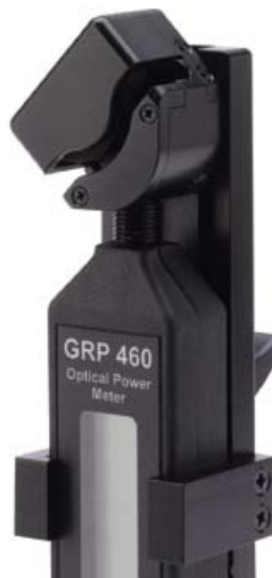
Adaptor GLFI 110 enables non intrusive detection of light on working fibres
