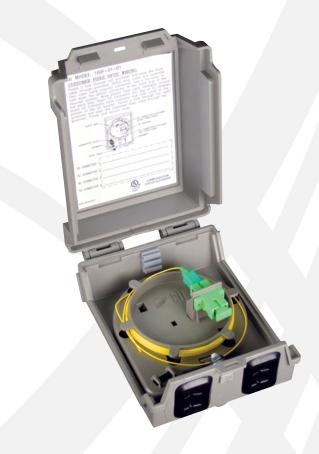
The FET1 is a compact enclosure which is designed to provide a demarcation and transition point between fiber drop cable and the customer premise fiber cable. Designed as an adapter plate for the Tii 169 Sealed Wire Terminal Enclosure, the unit can be factory installed with industry standard single, dual or quad fiber coupler(s). The internal fiber routing system allows for proper bend radius and slack storage of bend insensitive fiber.
