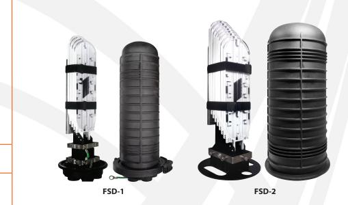
The Tii fiber optic splice enclosure is a butt end splice closure equipped with Roxtec cable sealing technologies. Constructed of superior materials to withstand harsh outdoor environments, such as UV degradation, chemical exposure and cold temperatures to ensure continuous operation of high speed fiber networks. The seals in the ports of the lid prevent gas, water or humidity from entering the enclosure.
